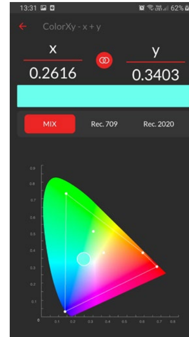
You can select 3 colors spaces on the xy mode: MIX (biggest space possible) REC709 and REC2020.
